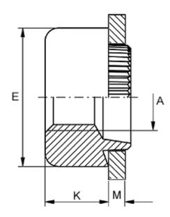
Female thread A = M2Height K = 3.0Outer diameter E = 8.0
